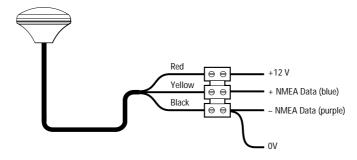
Figure 2-5 GPS Connections
